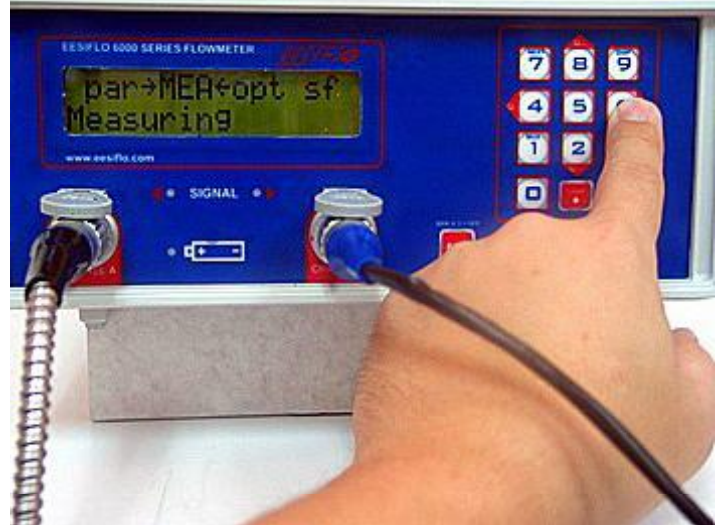
Step 27 Scroll back to Measuring. You should remove the thickness gage if you are not using it anymore.
