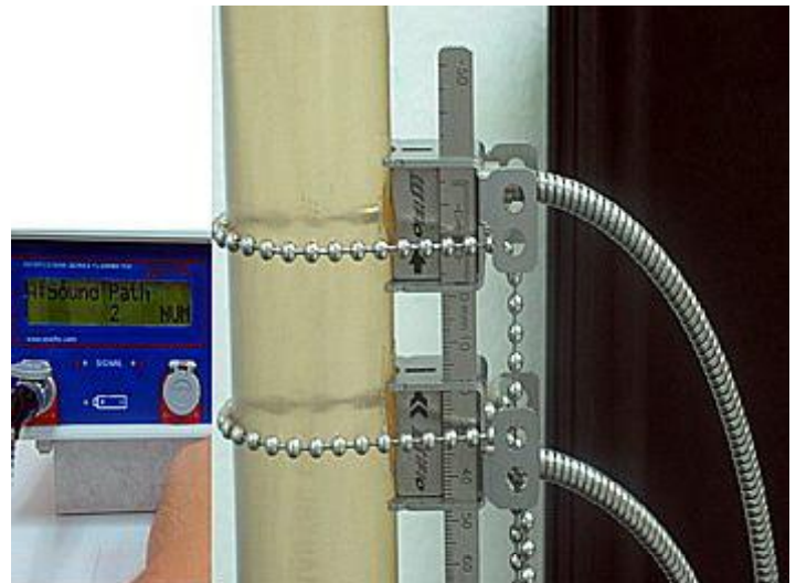
Step 29 Choose a Sound Path . In this case it is Sound path 2. The Transducers Should be on the same side of the pipe with arrows on the transducers pointing in the direction of the flow. You can find out more about other sound paths by referring to the user manual
