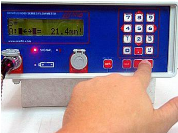
Step 34 If you have set up the flowmeter correctly, you will see the red signal light change to green and a display of signal strength on the screen
