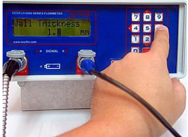
Step 16 Now go back to the Parameter for channel A and enter in the wall thickness
