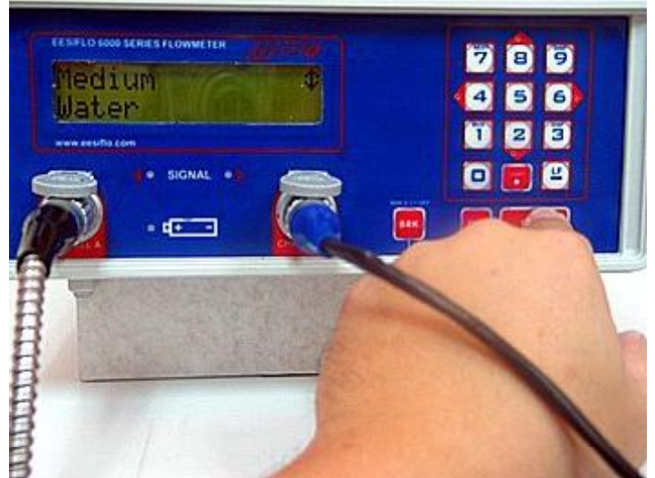
Step 20 Choose the Liquid you are Measuring from the Scroll down list
