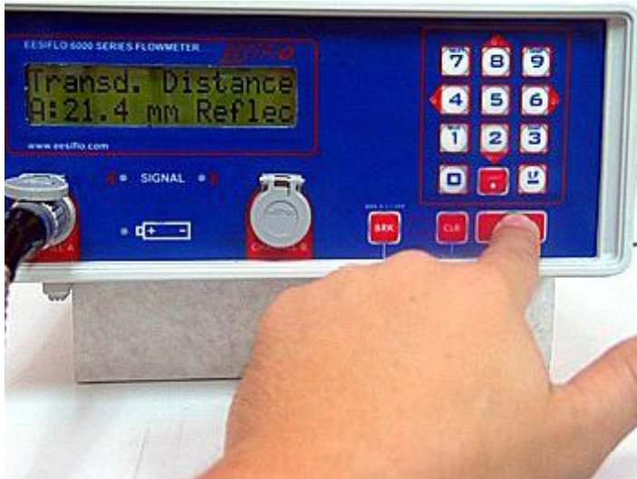
Step 30 The meter will tell you how far to space the transducers on the pipe
