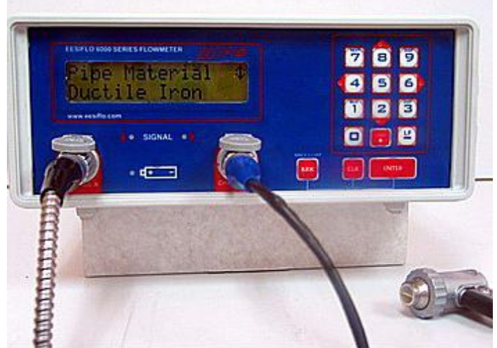
Step 10 If you don't know the wall thickness, you can use the optional thickness gauge to measure the pipe wall thickness .Or a thickness gauge from a reliable manufacturer. We would recommend you don't guess the wall thickness because it will affect the overall accuracy of your measurements.
