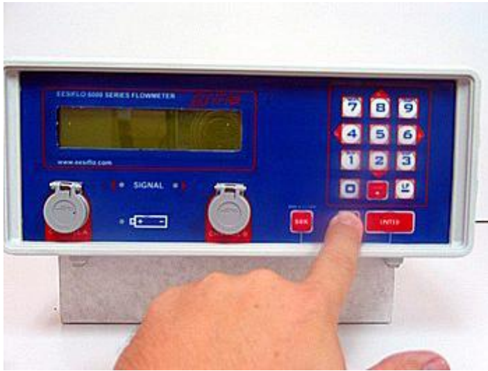
Step 1 Start by Turning the Power On. Use mains Power 110/220 VAC or The 15 hour battery
