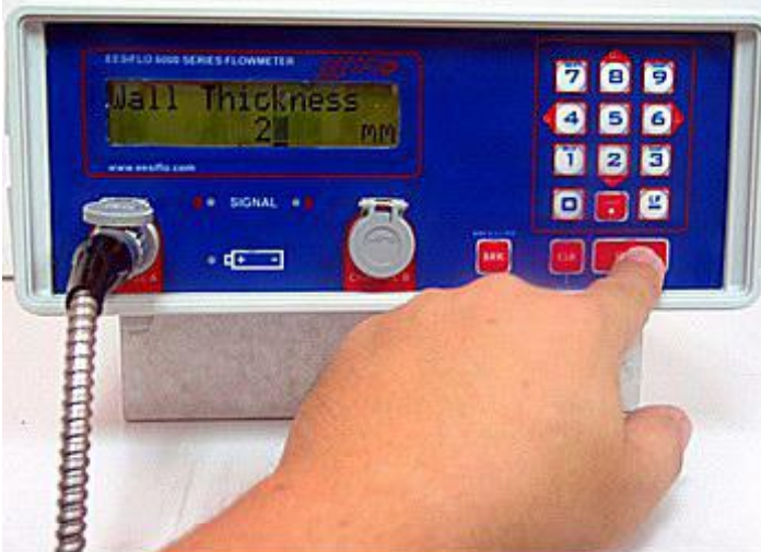
Step 9 Enter in the wall thickness
