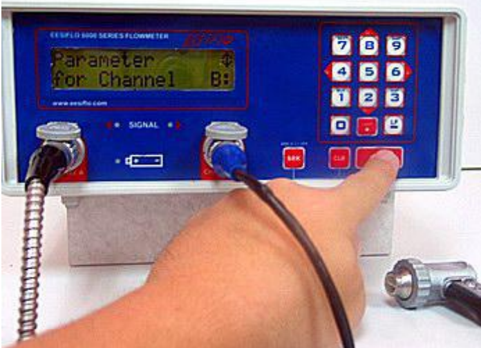
Step 11 In this case, scroll to the Parameter menu for Channel B since We plugged the gage into B
