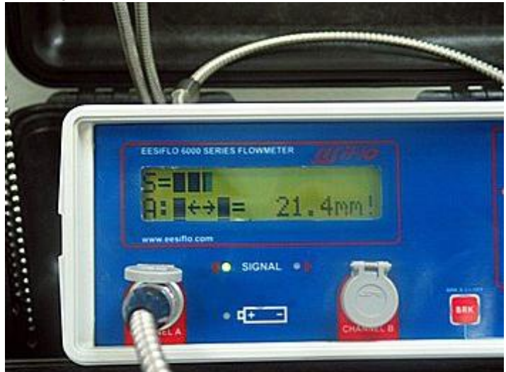
Step 34 If you have set up the flowmeter correctly, you will see the red signal light change to green and a display of signal strength on the screen
