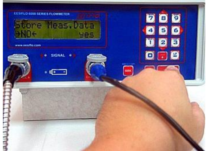
Step 26 The meter will ask you if you want to store data. In this case we are not. It will also ask if you want a serial output – again we are not using them in this example
