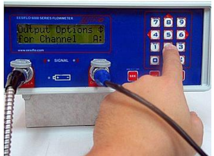
Step 22 Scroll to the Output options menu now to choose the Units of Measurement that you need
