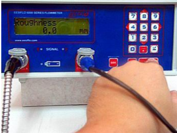
Step 19 Enter the Roughness of the Pipe or leave it at zero if you are not sure what it is
