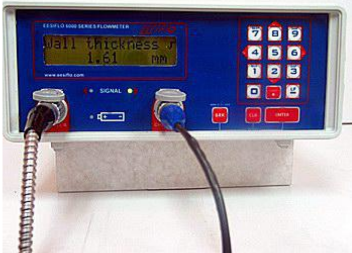
Step 15 When you see the Green Light, the display will show the wall thickness
