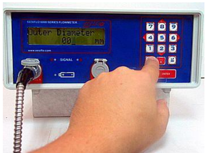
Step 6 If you know the pipe's outer diameter, enter it here. If you don't ,enter ZERO And press Enter
