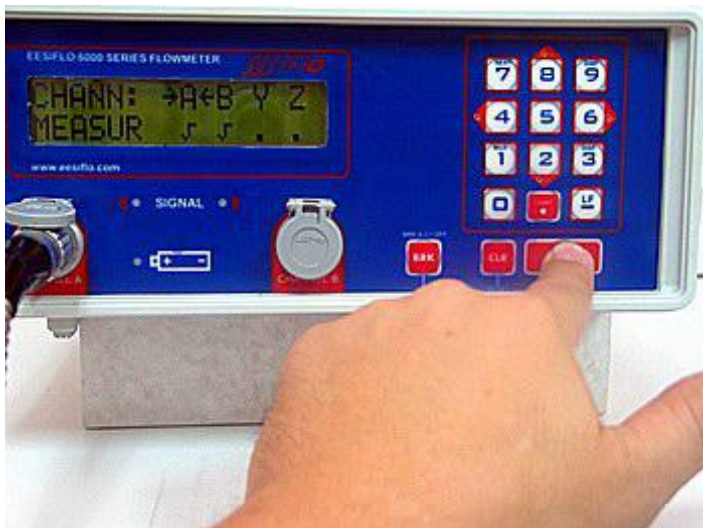
Step 28 You should choose channel A. Channel A is active when you See the square root sign under it.
