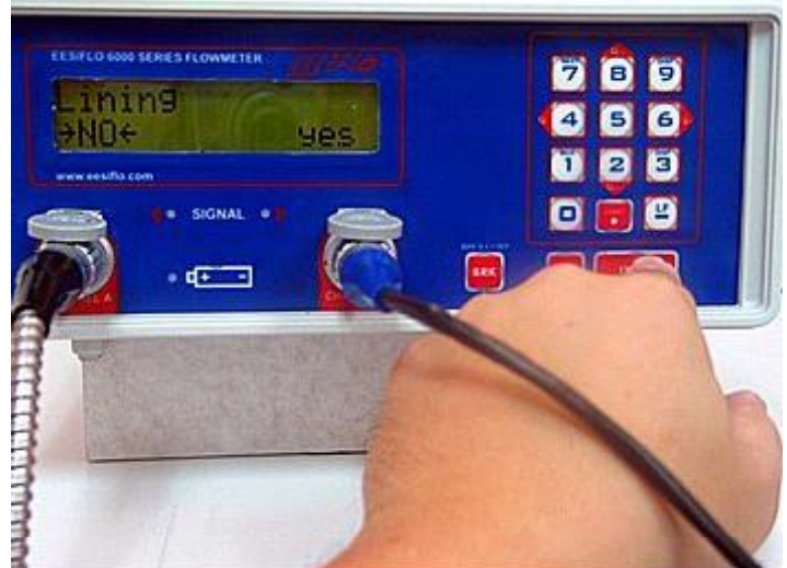
Step 18 Choose the Lining Material or Press NO if there is no liner in the pipe
