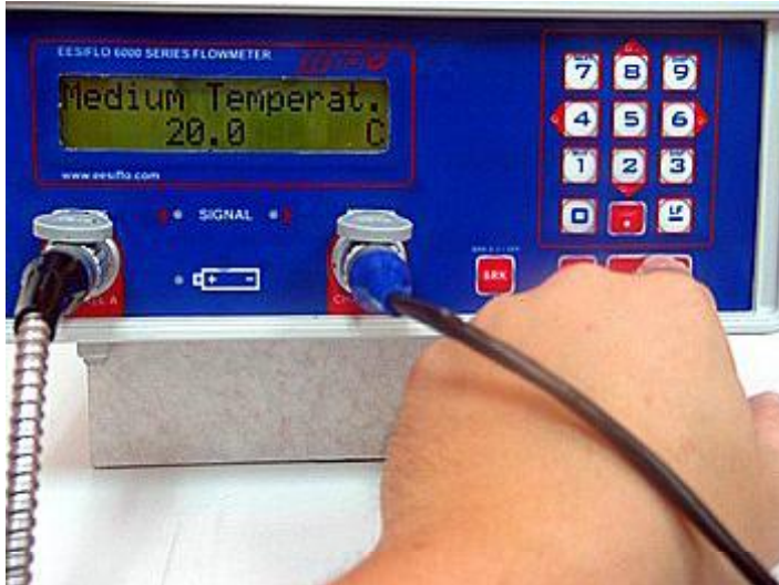
Step 21 Enter in the approximate liquid temperature
