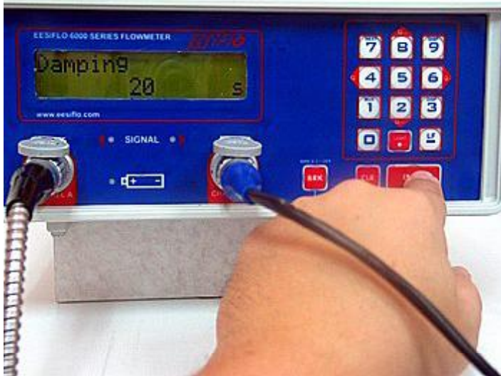
Step 25 Choose a Damping Time. If you don't know what this is, just leave it at 20
