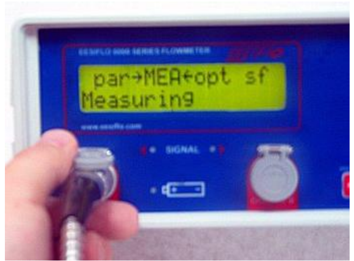
Step 2 Plug in the Transducers . EESIFLO 6000 will auto detect the transducers
