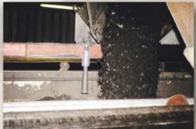
The KAB 20 Transducer is attached to a shuttle car and measures the level of the coal in the bunkers.
