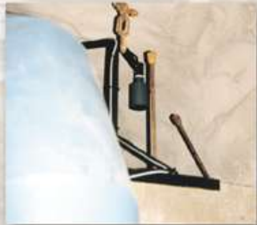
KAB 10 Transducer together with the SUMPI is being used to measure slurry 4 kilometers underground.
