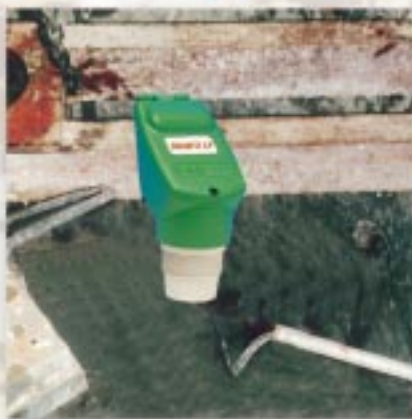
SHORTI LP measuring slurry, level being controlled by variable speed drive.
